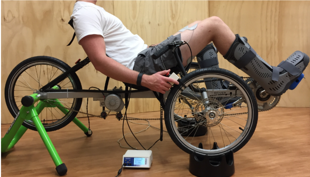
Figure 5-2. Motorized FES-cycling test bed. Photo courtesy of author.
