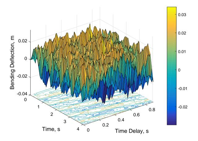
Figure 5-2. Closed loop bending deflection with constant input delays using the controller in [1].
