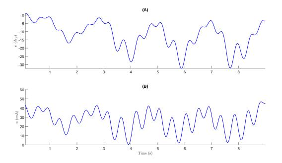
Figure 2-2. Tracking performance example taken from the right leg of subject 5 (S5-Right). Plot A illustrates the angle tracking error when  $\beta = 0$  in (2–9). Plot B depicts the control input (current amplitude in mA).
