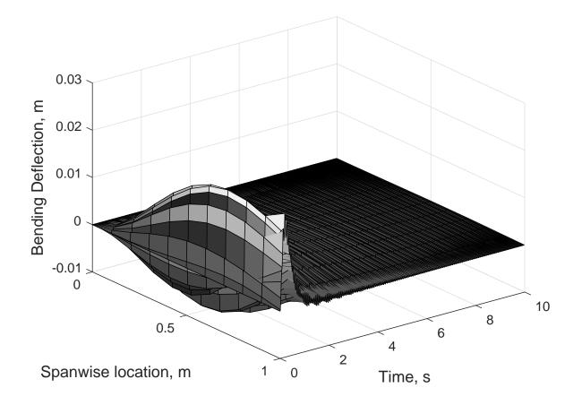
Figure 5-4. Bending deflection after applying the deigned controller in (5-23).
