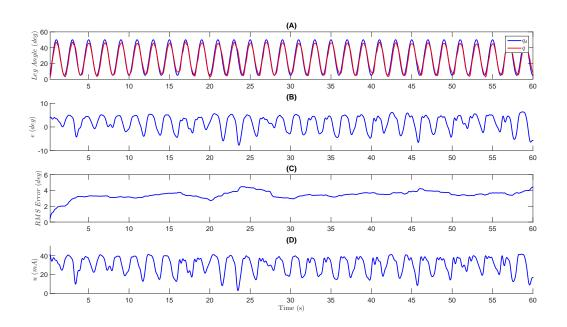
Figure 2-1. Tracking performance example taken from the right leg of subject 1 (S1-Right). Plot A includes the desired trajectory (blue solid line) and the actual leg angle (red line). Plot B illustrates the angle tracking error. Plot C depicts the RMS tracking error. Plot D depicts the control input (current amplitude in mA).
