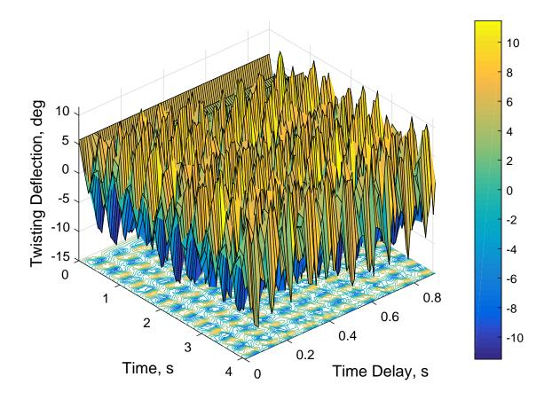
Figure 5-3. Closed loop twisting deflection with constant input delays using the controller in [1].
