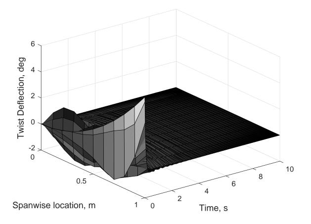
Figure 5-5. Twisting deflection after applying the deigned controller in (5-23).
