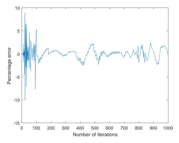
Figure 3-2. Delay mismatch variation with training iteration.
