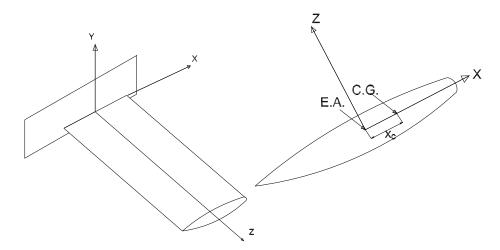
Figure 5-1. Schematic of the wing section, where E.A. denotes the elastic axis and C.G. denotes the center of gravity..
