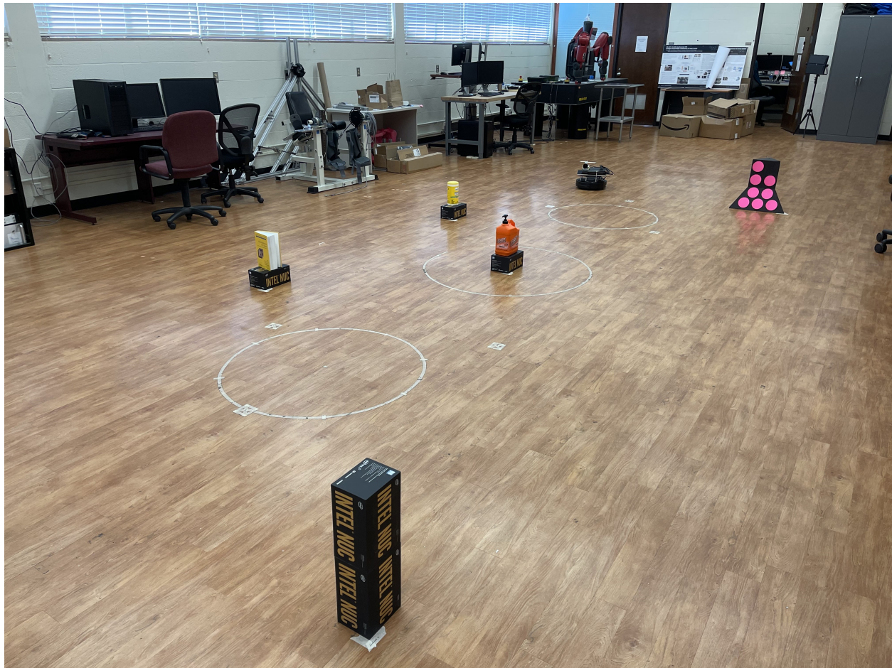
Figure 3-1. The experimental setup using one WMR with an onboard monocular camera and five customized landmarks. The centroid of each landmark is at the center of a feedback available region, and the radius of each feedback available region is selected as 0.8 m. The WMR can obtain pose estimates (i.e., true state information) when one of the landmarks is within the FOV of the monocular camera.
