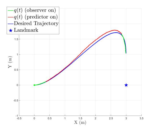
Figure 2-2. The trajectory tracking result. The green and red trajectories indicate whenever the observer and predictor are activated, respectively. When the predictor is active, the WMR diverges from the desired trajectory because of the disturbance. However, when the landmark returns to the FOV, regulation of the tracking error is achieved.
