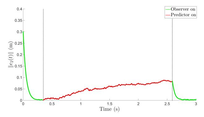
Figure 2-4. State estimation error. The estimate is exponentially regulated to the true state whenever the observer is active and diverges whenever the predictor is active.
