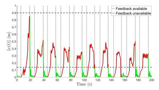
Figure 4-2. The evolution of ||e(t)|| for continuous state estimates. The tracking error is regulated below  $\hat{e}_T$  (bottom dotted line) before leaving  $\mathcal{F}$  and remains under  $e_M$  (top dotted line) for all times when outside of  $\mathcal{F}$ . The vertical lines denote the instants when x(t) enters and leaves  $\mathcal{F}$ .
