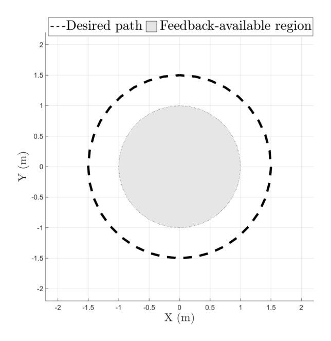
Figure 3-3. A representation of the feedback-available region and the desired path. The gray region denotes the feedback-available region, which is 1.0 meter in radius, and the black dotted line denotes  $x_d$ , which is a circular path with a radius of 1.5 meters.
