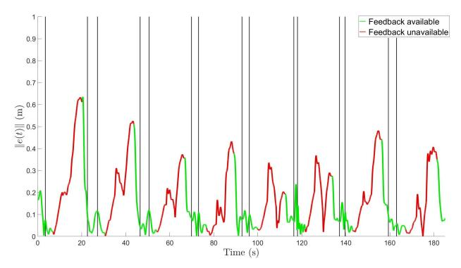
Figure 3-8. Actual tracking error ||e(t)||. The dash-dot lines indicate the switching interface of minimum and maximum dwell times.
