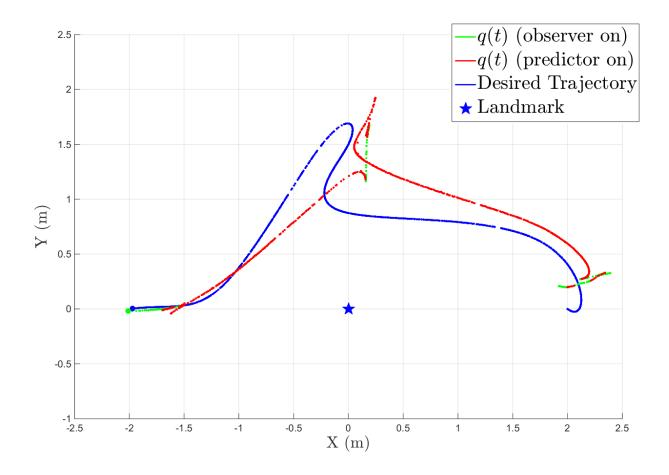
Figure 2-5. The trajectory tracking result. The green and red trajectories indicate whenever the observer and predictor are activated, respectively. When the predictor is active, the WMR diverges from the desired trajectory because of the disturbance. However, when the landmark returns to the FOV, the WMR adjusts its course to compensate for the accumulated error.
