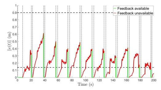
Figure 4-4. The evolution of ||e(t)|| for discrete state estimates using a reset map. The tracking error is regulated below  $\hat{e}_T$  (bottom dotted line) before leaving  $\mathcal{F}$  and remains under  $e_M$  (top dotted line) for all times when outside of  $\mathcal{F}$ . The vertical lines denote the instants when x(t) enters and leaves  $\mathcal{F}$ .
