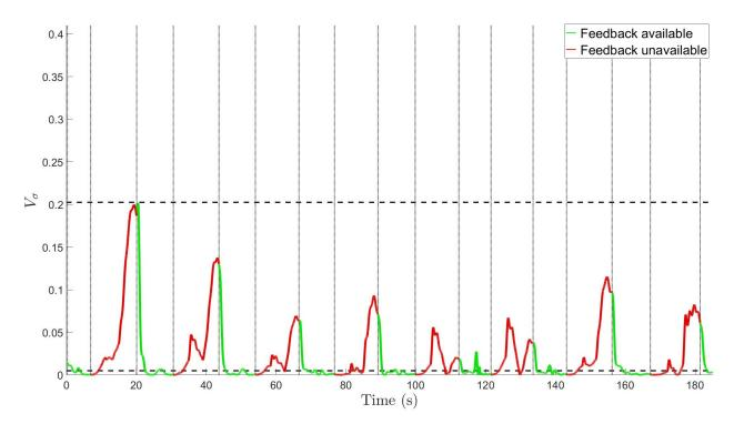
Figure 3-9. Evolution of  $V_{\sigma}(t)$ . The dotted (vertical) lines indicate the time instants when the quadcopter crossed the feedback region boundary. The dashed (horizontal) lines indicate the prescribed  $V_M$  and  $V_T$  for  $V_{\sigma}$ .
