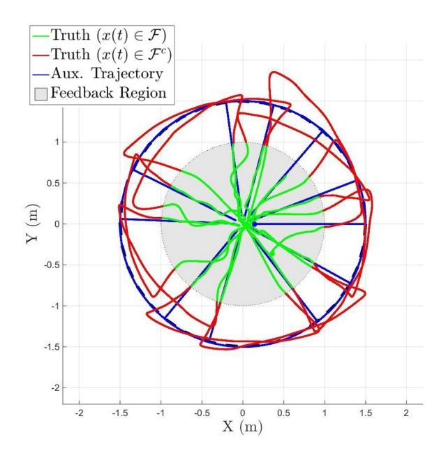
Figure 4-1. Overall path following result using an observer for the state estimate. The agent is required to remain inside the feedback-available region for periods of time as indicated by the green line.
