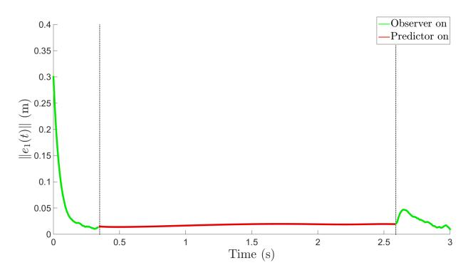
Figure 2-3. State estimate tracking error. The estimate tracking error is regulated when the predictor is activated because the update law propagates the state estimate using a model of the WMR. When the observer is activated at 2.6 secs, the estimate initially converges towards the true state and eventually converges to the desired trajectory along with the true state.
