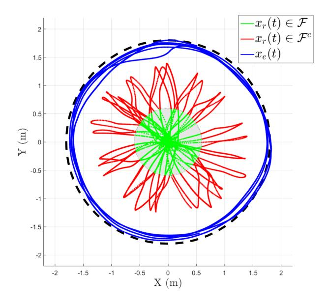
Figure 5-2. The overall tracking result for the relay and exploring agent. The green and red lines denote the trajectories of the relay agent when inside and outside the feedback-available region, respectively. The blue line represents the trajectory of the exploring agent, which is initialized at (0.5, 1.7).
