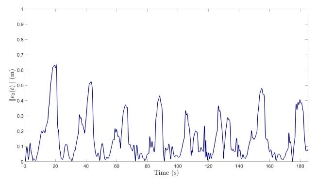
Figure 3-6. Estimation error  $||e_2(t)||$ . As indicated by the analysis, the estimation error converges when  $x(t) \in \mathcal{F}$  and diverges when  $x(t) \in \mathcal{F}^c$ .
