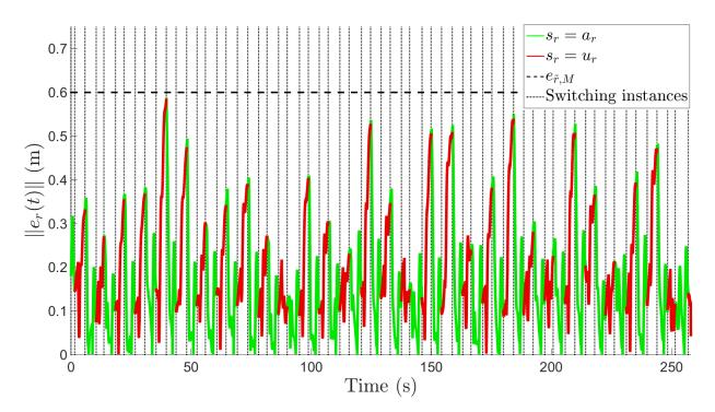
Figure 5-5. The tracking performance plot for  $||e_r(t)||$ . The green and red trajectories denote the change in  $||e_r(t)||$  when the relay agent is inside and outside the feedback-available region, respectively. The vertical dotted lines denote the time instances when the relay agent crosses the boundaries of the feedback-available region (i.e.,  $t_{r,i}^a$  and  $t_{r,i}^u$ ).
