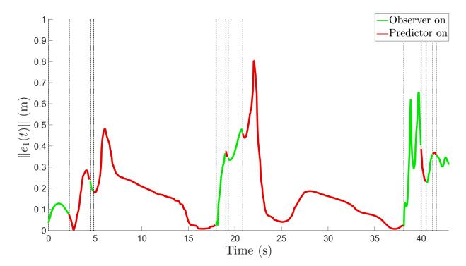
Figure 2-6. State estimate tracking error. During the periods of time between 5 to 18 seconds and 21 to 38 seconds, the estimate tracking error is regulated because the predictor update law propagates the state estimate using a model of the WMR. When the observer is active, the state estimate is regulated towards the true state, and hence, the estimate tracking error may increase.
