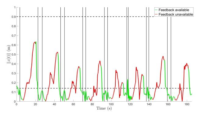
Figure 3-7. Evolution of ||z(t)||. The dash-dot (vertical) lines indicate the switching interface of minimum and maximum dwell times, and the dashed (horizontal) lines indicate the prescribed upper bound and lower threshold.
