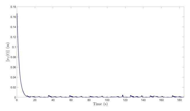
Figure 3-5. Estimate tracking error  $||e_1(t)||$ . As indicated by the analysis, the estimate tracking error exhibits exponential stability regardless of feedback availability.
