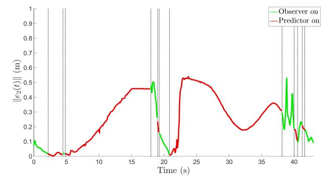
Figure 2-7. State estimation error. When the predictor is active for a prolonged period of time, the stability of the estimation error is not guaranteed. When the observer is active, estimation error is regulated.
