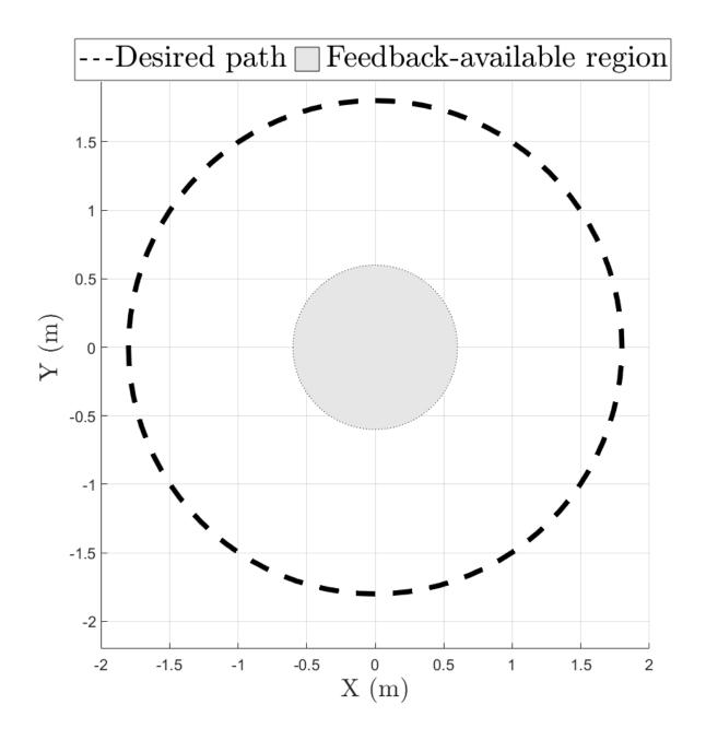
Figure 5-1. A representation of the experimental setup. The gray region denotes the feedback-available region, which is 0.6 meters in radius, and the black dotted line denotes  $x_d$ , which is a circular path with a radius of 1.8 meters. As a comparison, the ratio between the radius of the desired path and the feedback-available region is 300%, versus 150% in Chapter 4 (1 meter radius for the feedback-available region and 1.5 meters for the desired circular path).
