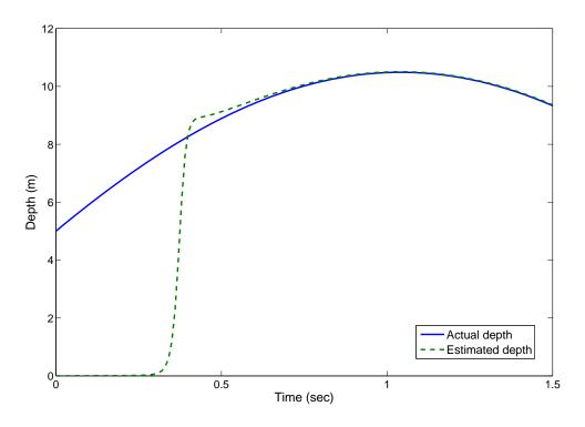
Figure 3-6. Depth estimation with large initial condition  $\alpha(t_0) = 300$  using the proposed observer.
