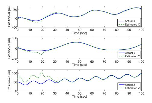
Figure 5-7. Comparison of the actual and estimated 3D relative position of the object and the camera for time-varying object velocity  $v_p(t)$ .
