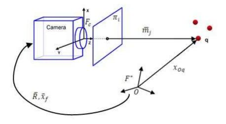
Figure 2-2. Moving camera looking at the static scene.
