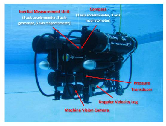
Figure 3-8. AUV experimental setup.
