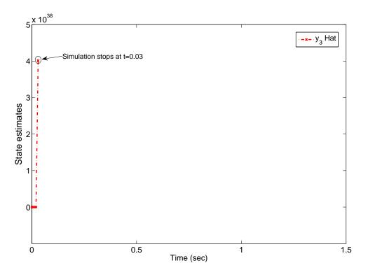
Figure 3-7. State estimation using the observer in [2] for large initial conditions. Since the state estimate is very large, simulation fails to integrate at t = 0.03.
