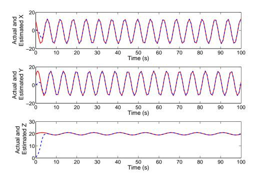
Figure 7-1. Comparison of the actual and estimated X,Y and Z positions of a moving object with respect to a moving camera.
