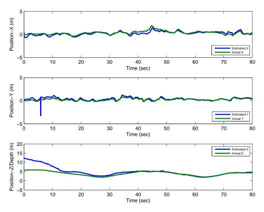
Figure 3-10. Comparison of the estimated and ground truth range of the buoy with respect to the underwater vehicle.
