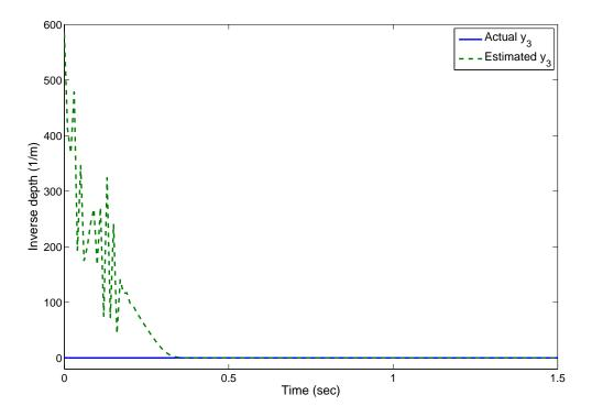
Figure 3-5. Estimation of  $\hat{y}_3(t)$  starting from large initial condition  $\alpha(t_0) = 300$  using the proposed observer.
