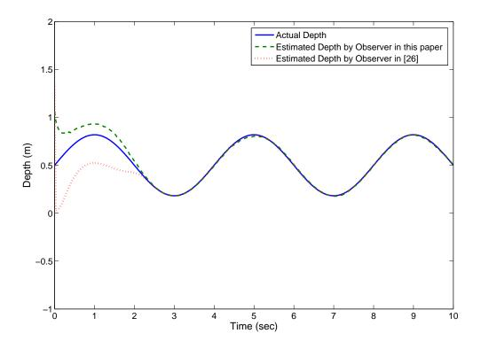
Figure 3-2. Comparison of the depth estimation using the proposed observer and the observer in [2] when camera motion does not satisfy Assumption 3.1.
