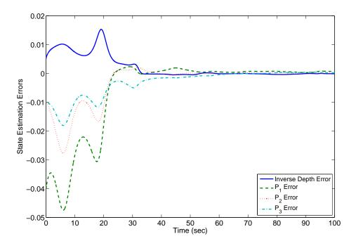
Figure 5-6. State estimation errors for time varying velocity,  $v_{p}\left(t\right)$ , using the proposed observer.
