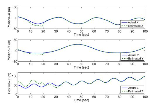
Figure 5-4. Comparison of the actual and estimated 3D relative position of the object and the camera.
