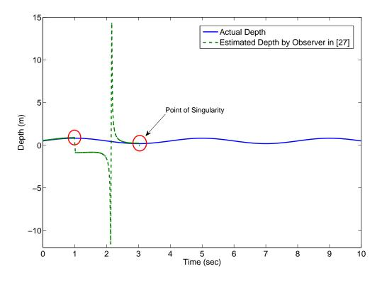
Figure 3-4. Depth estimation using the observer in [1].
