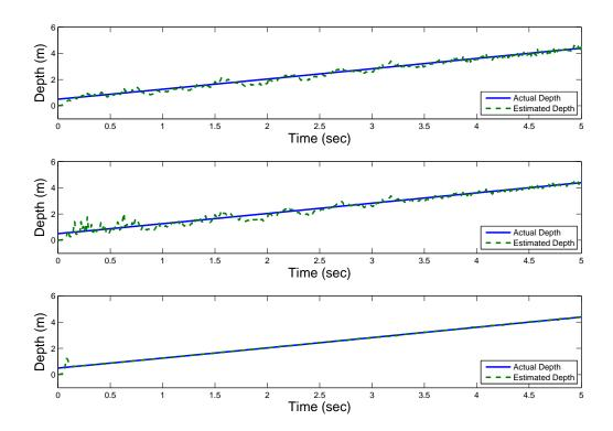
Figure 3-1. Comparison between the true and estimated depth in the presence of measurement noise A) top subplot shows the estimated depth using the proposed observer. B) middle subplot shows the estimated depth using the observer in [1]. C) bottom subplot shows the estimated depth using the observer in [2].
