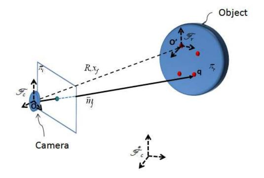
Figure 2-1. Coordinate frame relationships of a moving camera and an object.
