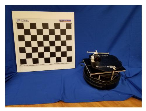
Figure 3-1. Photo courtesy of author. Image shows the checkerboard, Kobuki Turtlebot, and an iDS uEye camera used for experiments.
