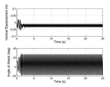
Figure 3-1. Aeroelastic system open-loop response without disturbances
