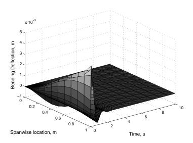
Figure 4-6. Closed-loop bending deflection of the flexible aircraft wing.
