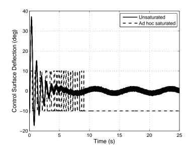
Figure 3-3. Commanded control effort for the controller developed in [2] with and without an *ad hoc* saturation.
