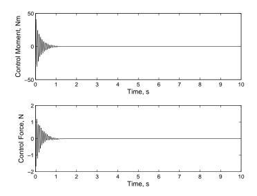
Figure 4-8. Lift and Moment commanded at the wing tip.
