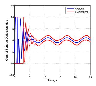
Figure 3-8. Control surface deflection for all 1500 Monte Carlo samples. The control effort for all samples remain within the actuation limit and demonstrate similar steady state performance.
