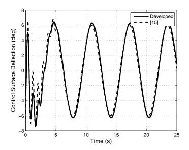
Figure 2-6. Control surface deflection,  $\delta(t)$ , for the developed controller and the controller from [15]
