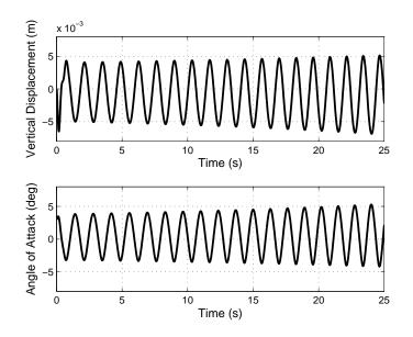
Figure 2-2. Aeroelastic system free response without disturbances
