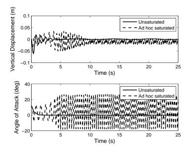
Figure 3-2. State trajectories of the controller developed in [2] with and without an *ad hoc* saturation.
