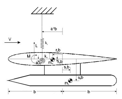
Figure 2-1. Diagram depicting the two degree of freedom airfoil section with attached store based on that in [1].
