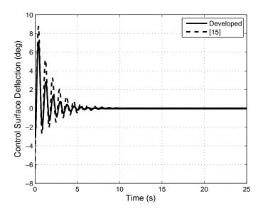
Figure 2-4. Control surface deflections,  $\delta(t)$ , for the developed controller and the controller from [15]
