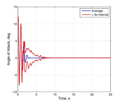
Figure 3-6. AoA trajectories for all 1500 Monte Carlo samples. The developed saturated controller suppressed the LCO behavior in all samples and the majority of the samples exhibit similar transient performance.
