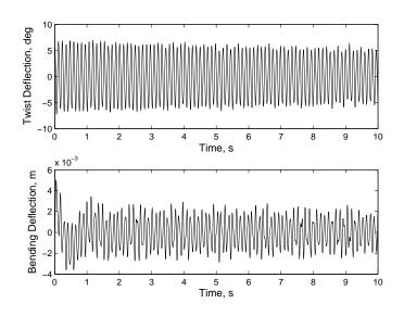
Figure 4-4. Open-loop response at the wing tip of the flexible aircraft wing.
