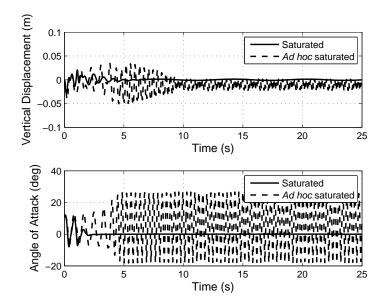
Figure 3-4. Comparison of the closed-loop aeroelastic system response of the controller in [2] with an *ad hoc* saturation and the developed saturated controller.
