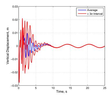
Figure 3-7. Vertical position trajectories of all 1500 Monte Carlo samples. The vertical position remained bounded for all samples despite being an uncontrolled state.
