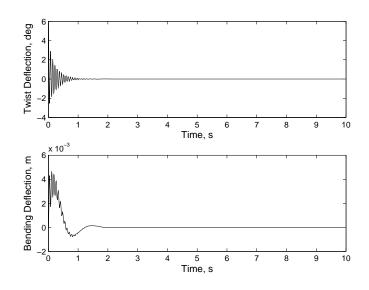
Figure 4-7. Closed-loop response at the wing tip of the flexible aircraft wing.
