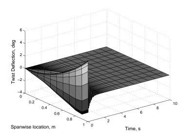
Figure 4-5. Closed-loop twist deflection of the flexible aircraft wing.
