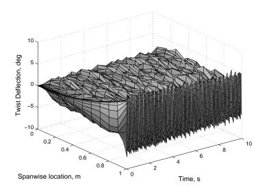
Figure 4-2. Open-loop twist deflection of the flexible aircraft wing.
