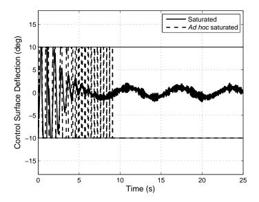
Figure 3-5. Comparison of the control surface deflections for the developed saturated controller and *ad hoc* saturated controller from [2]
