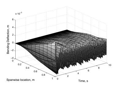
Figure 4-3. Open-loop bending deflection of the flexible aircraft wing.
