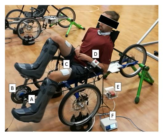
Figure 2-1. Motorized FES cycle: (A) Encoder (B) Power Meter (C) Electrodes (D) E-Stop (E) Filter Card (F) Stimulator.
