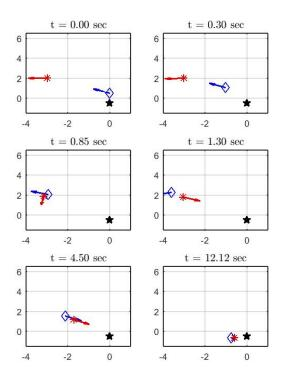
Figure 6-4. Sampled positions of the influencing and roaming agents. The influencing agent (blue diamond) intercepts and drives the roaming agent (red asterisk) to the desired state (black star).
