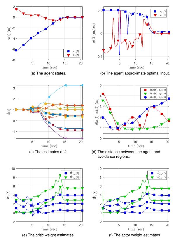
Figure 4-6. The states, control policy, and weight estimates of the agent are shown in addition to the distances between the agent and each avoidance region center for the third experiment.
