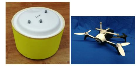
Figure 5-3. The unactuated paper platform (left) representing the roaming agent, and the Parrot Bebop 2.0 quadcopter (right) representing the influencing agent.
