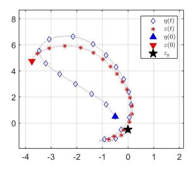
Figure 5-2. Positions of the influencing and roaming agents. The influencing agent (blue diamonds) intercepts and regulates the roaming agent (red stars) to the goal location (black star). The initial influencing agent condition is given by the blue triangle and the initial roaming agent condition is given by the red triangle.
