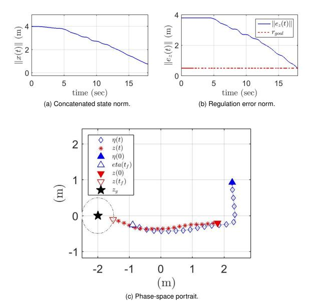
Figure 5-5. The (a) concatenated state norm, ||x(t)||, (b) regulation error norm,  $||e_z(t)||$ , and (c) phase-space portrait for experiment nine. In Figure 5-5c, the influencing agent (blue diamonds) regulates the roaming agent (red stars) to a neighborhood ( $r_{goal} = 0.5$  m) of goal location (black star). The initial influencing agent condition is given by the blue triangle and the initial roaming agent condition is given by the red triangle.
