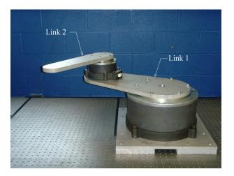
Figure 2-7. The experimental testbed consists of a two-link robot. The links are mounted on two NSK direct-drive switched reluctance motors.
