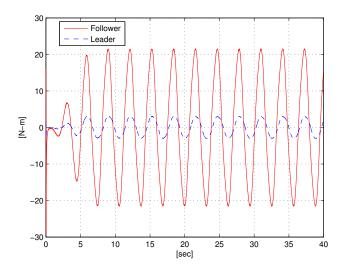
Figure 3-2. The simulated torques for the RISE and Stackelberg optimal controller.
