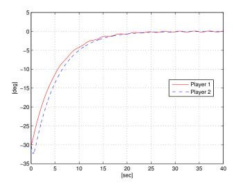
Figure 2-1. The simulated tracking errors for the RISE and Nash optimal controller.
