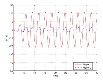
Figure 2-2. The simulated torques for the RISE and Nash optimal controller.
