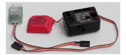
Figure B–6: Eagle Tree, Seagull, Wireless Dashboard Flight System - Pro Version: (1) Wireless Telemetry Transmitter, (2) Eagle Tree Systems G-Force Expander, and (3) Eagle Tree Systems GPS Expander
