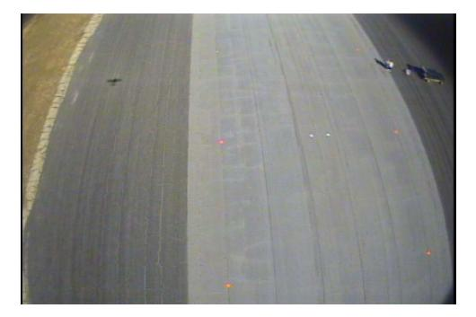
Figure 4–13: Single video frame from second flight test experiment illustrating the effect of the more forward looking, wider field of view camera.
