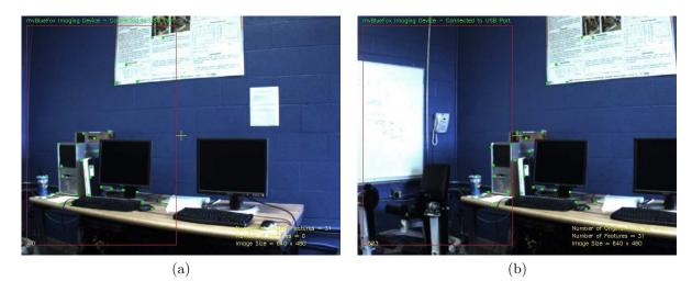
Figure 2-1. Two views of a scene and the matched feature points between the images.
