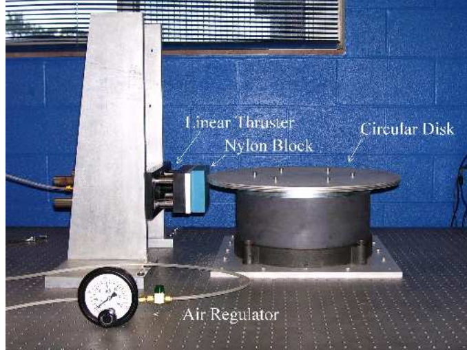
Figure 2-1. The experimental testbed consists of a circular disk mounted on a NSK direct-drive switched reluctance motor.
