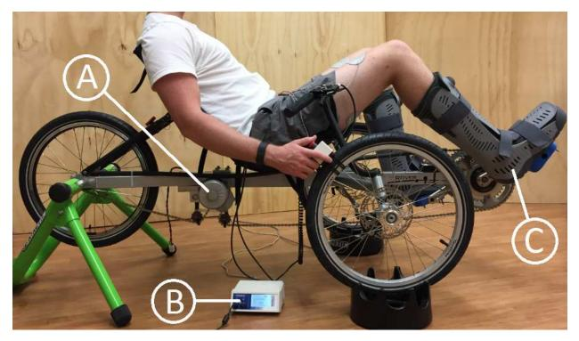
Figure 5-1. The motorized FES-cycling test bed used for experiments, consisting of (A) an electric motor, (B) stimulator, and (C) orthotic pedals. Photo courtesy of Matthew Bellman. Gainesville, FL.
