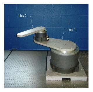
Figure 5-1. Experimental testbed consisting of a 2-link robot. The input delay in the system was artificially inserted in the control software.
