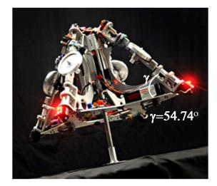
Figure 2-1. The University of Florida control moment gyroscope experimental test bed.
