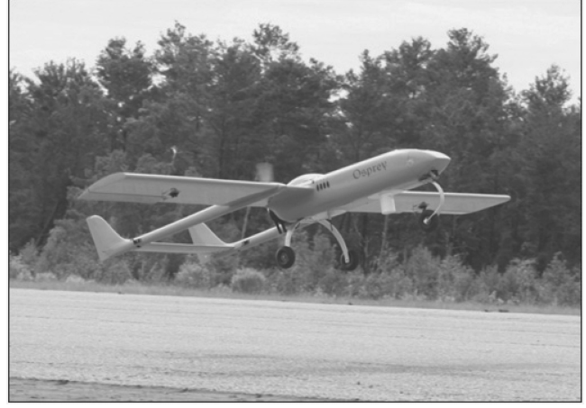
Fig. 4. Air and Sea Inc. Osprey UAV used in experiments and modeled for simulations.
