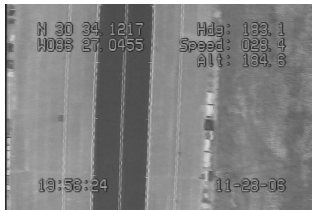
Fig. 14. Single video frame with GPS overlay illustrating landmarks placed along inside edge of runway.
