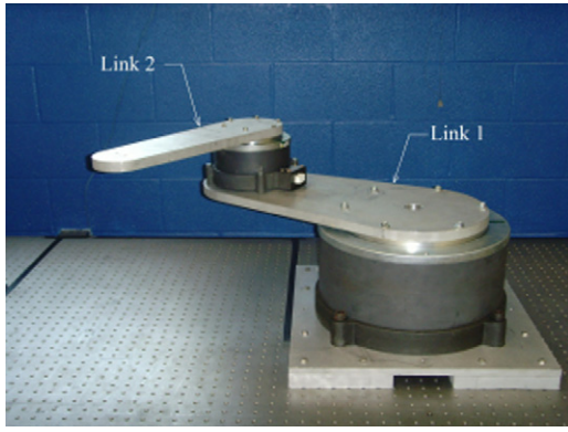
Fig. 1. Experimental testbed consisting of a two-link robot. The input delay in the system was artificially inserted in the control software.
