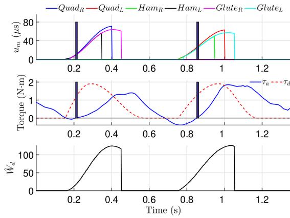
**Fig. 2.** FES intensities  $u_m$  (top), active torque output  $\tau_a$  and desired torque  $\tau_d$  (middle), and RLC input  $\dot{W}_d$  (bottom) during a single crank cycle for participant S3 after 2 min of cycling. The vertical solid bars correspond to the time where the torque output rises above zero, which illustrates the fact that muscle activation is affected by the muscle electromechanical delay (EMD) (Downey, Merad, Gonzalez, & Dixon, 2017).
