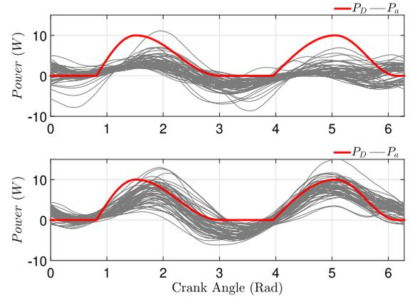
**Fig. 5.** Active power  $P_a$  and desired power  $P_d$  as a function of the crank angle for a trial with peak power  $P_d = 10$  W and desired cadence  $\dot{q}_d = 50$  RPM during the first 50 (top) and the subsequent 50 (bottom) crank cycles for participant S3.
