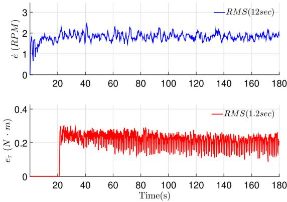
**Fig. 3.** Tracking performance for participant B quantified by the RMS cadence tracking error  $\dot{e}$  computed with a moving time interval window of 12 s (top), and the RMS torque tracking error  $e_\tau$  computed with a moving time interval window of 1.2 s (bottom).
