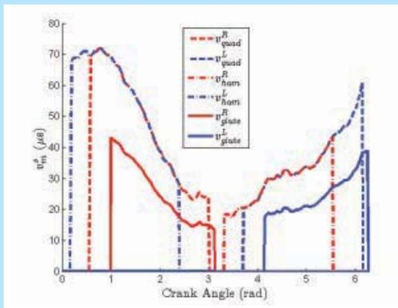
**FIGURE 2** Stimulation pulse width for each muscle group for a healthy normal person as a function of the crank cycle.
