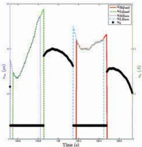
**FIGURE 4** Stimulation pulse width (denoted by  $u_m$  in microseconds) and motor control (denoted by  $u_e$  in amps) inputs for the quadriceps and hamstring muscle groups and an electric motor for an example healthy normal individual.
