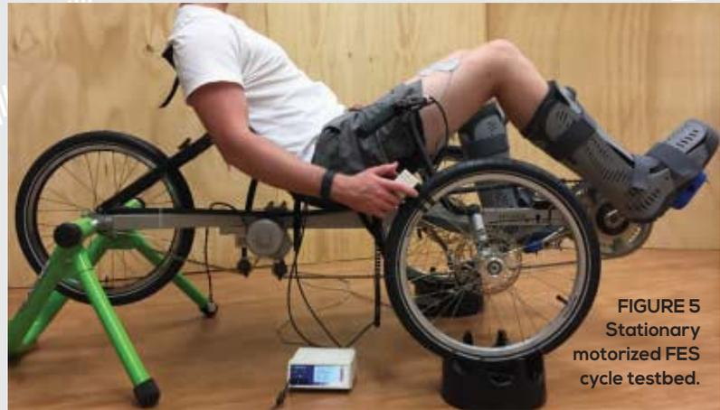
**FIGURE 5** Stationary motorized FES cycle testbed.
