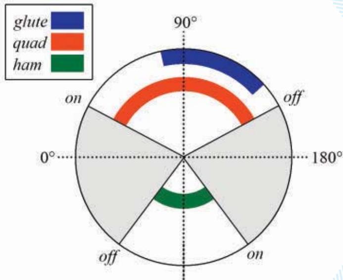
**FIGURE 1** Example stimulation pattern as a function of the crank position for the gluteal, quadriceps, and hamstring muscle groups on a single leg. Grey shaded regions indicate sections of the crank cycle where it is inefficient for a selected muscle group to produce torque. Electrical stimulation is turned on and delivered to respective muscles in specified regions and turned off in regions where it is inefficient to produce torque.
