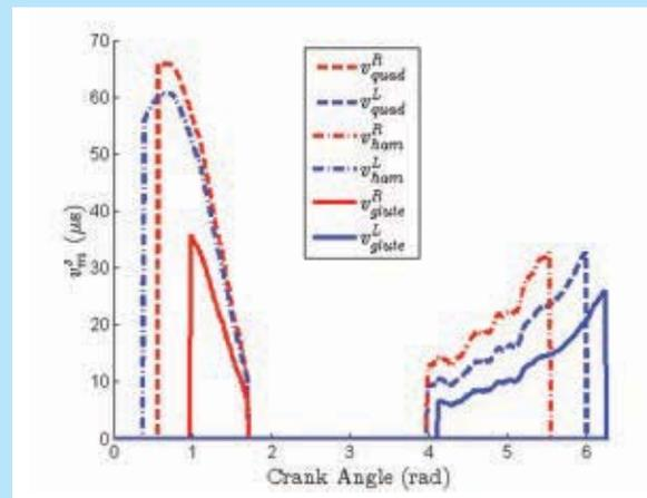
**FIGURE 3** Stimulation pulse width for each muscle group as a function of the crank cycle for an individual with decreased strength in the right side due to Parkinson's disease.
