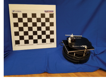
Fig. 2. Image shows the checkerboard, Kobuki Turtlebot, and iDS uEye camera used for experiments.
