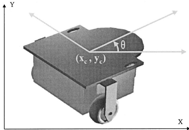
Fig. 1 Two-dimensional kinematic wheel
