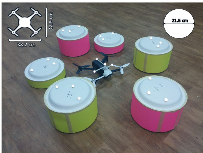
Fig. 12. Parrot Bebop 2 quadcopter used for the herder as well as the paper platforms that represent the targets is shown. The markers seen on each agent are infrared reflectors arranged in unique configurations, which are used with the NaturalPoint, Inc. OptiTrack motion capture system to track the positions of each agent for feedback control at 120 Hz. Each target agent platform has a different height and weight, and are designed to slide without tipping on the floor shown.
