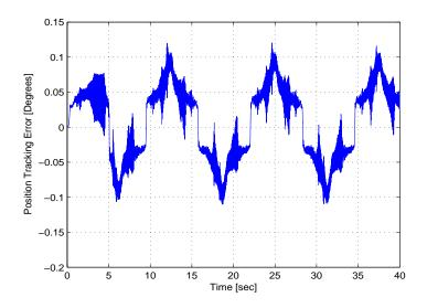
Figure 3–3: Position tracking error from the model-based controller with friction feedforward terms as described in (3–40).
