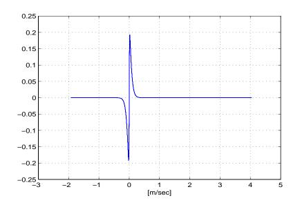
Figure 2–13: Friction coefficient vs slip velocity.
