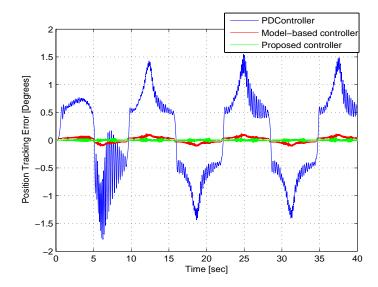
Figure 3–5: Comparison of position tracking errors from the three control schemes.
