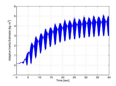
Figure 4–7: Parameter estimate for the mass of the link assembly.
