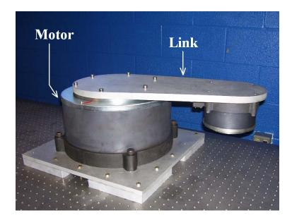
Figure 4–1: The experimental testbed consists of a 1-link robot mounted on a NSK direct-drive switched reluctance motor.
