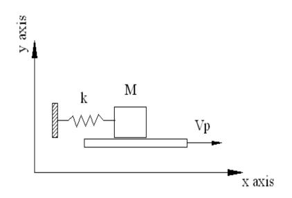
Figure 2–4: Mass-spring system for demonstrating stick-slip friction.
