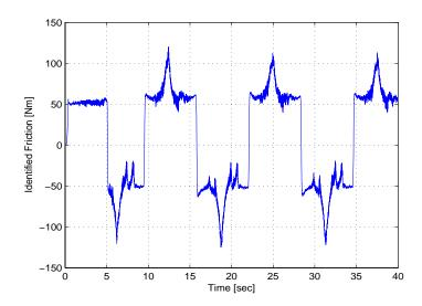
Figure 3–22: Identified friction from the adaptive term in the proposed controller when the circular disk was lubricated.
