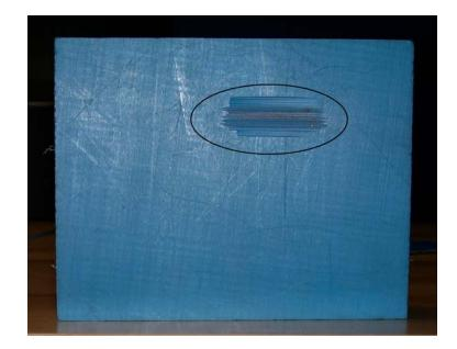
Figure 3–26: Wearing of the Nylon block where it rubbed against the circular disk.
