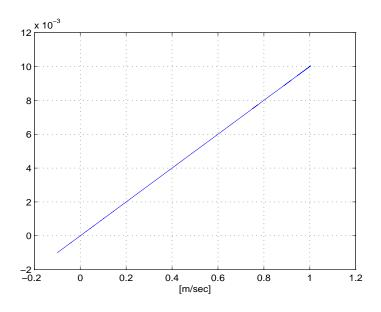
Figure 2–9: Friction coefficient vs slip velocity.
