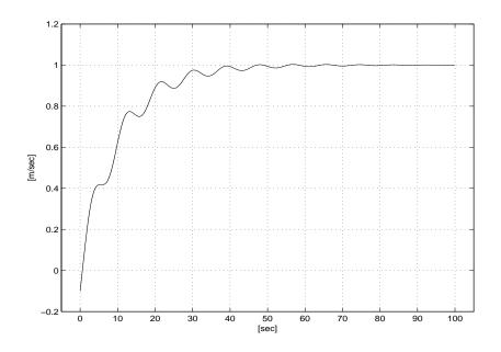
Figure 2–11: Slip velocity vs time.
