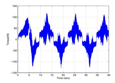
Figure 3–8: Torque input by the model-based controller with friction feedforward terms as described in (3–40).
