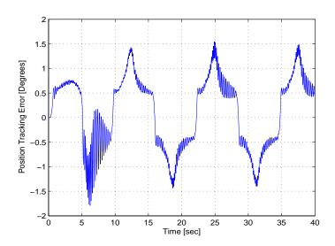
Figure 3–2: Position tracking error from the PD controller.
