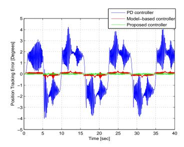
Figure 3–14: Comparison of position tracking errors from the three control schemes.
