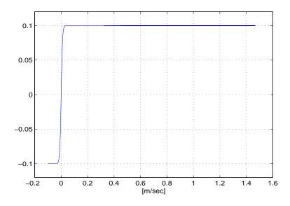
Figure 2–5: Friction coefficient vs slip velocity.
