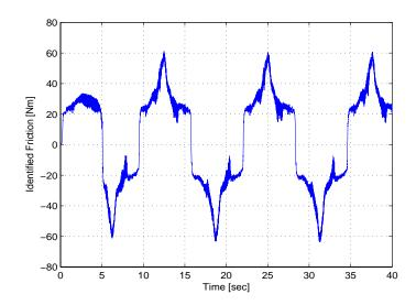
Figure 3–10: Identified friction from the adaptive term in the proposed controller.
