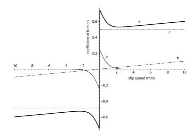
Figure 2–1: Friction model as a composition of different effects including: a) Stribeck effect, b) viscous dissipation, c) Coulomb effect, and d) the combined model.
