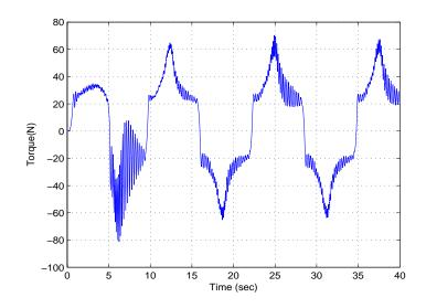
Figure 3–7: Torque input by the PD controller.
