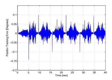
Figure 3–20: Position tracking error with the proposed controller when the circular disk was lubricated.
