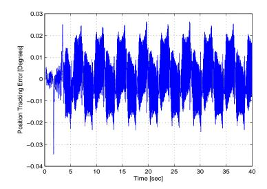
Figure 4–3: Position tracking error when the adaptive gain is zero.
