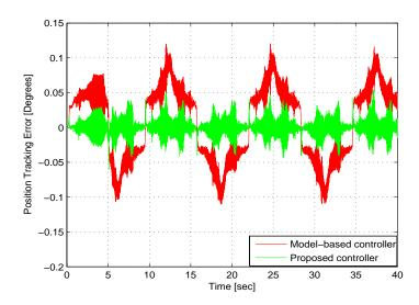
Figure 3–6: Comparison of position tracking errors from the model-based controller and the proposed controller.
