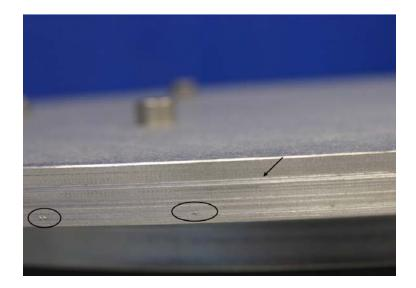
Figure 3–27: Wear on the circular disk.
