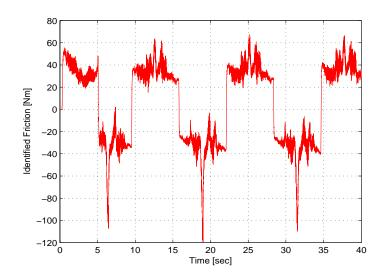
Figure 3–23: Net external friction induced with no lubrication. The net friction was calculated by subracting the identified friction term in Experiment 1 from the identified friction term in Experiment 2.
