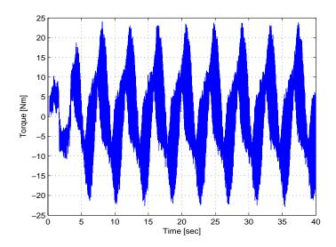
Figure 4–4: Torque input when the adaptive gain is zero.
