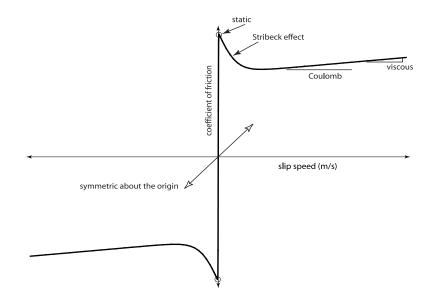
Figure 2–2: Characteristics of the friction model.
