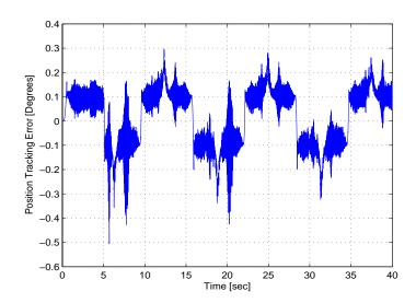
Figure 3–12: Position tracking error from the model-based controller with friction feedforward terms as described in (3–40).
