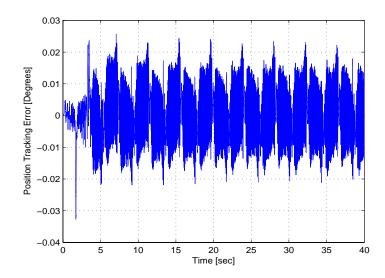
Figure 4–5: Position tracking error for the control structure that includes the adaptive update law.
