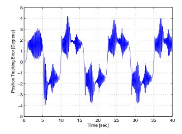
Figure 3–11: Position tracking error from the PD controller.
