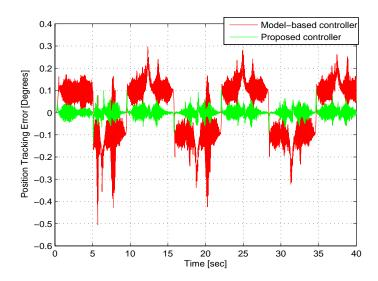
Figure 3–15: Comparison of position tracking errors from the model-based controller and the proposed controller.
