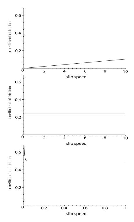
Figure 2–3: Modular ability of the model to selectively model different friction regimes: top plot-viscous regime (e.g., hydrodynamic lubrication), middle plot-Coulombic friction regime (e.g., solid lubricant coatings at moderate sliding speeds), and bottom plot-abrupt change from static to kinetic friction (e.g., non-lubricous polymers).
