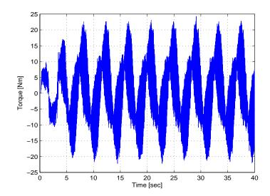
Figure 4–6: Torque input for the control structure that includes the adaptive update law.
