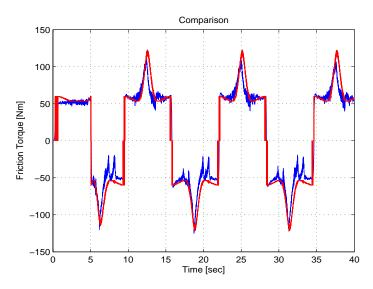
Figure 3–25: The friction torque calculated from the model in (2–1) approximates the experimentally identified friction torque in (3–9).
