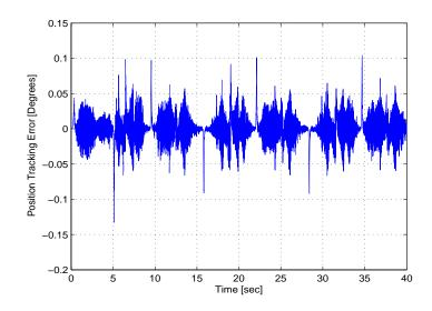
Figure 3–13: Position traking error from the proposed controller.
