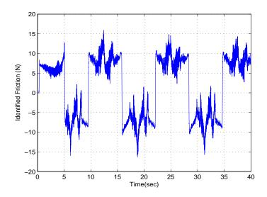
Figure 3–24: Net external friction induced with lubrication. The net friction was calculated by subracting the identified friction term in Experiment 1 from the identified friction term in Experiment 3.
