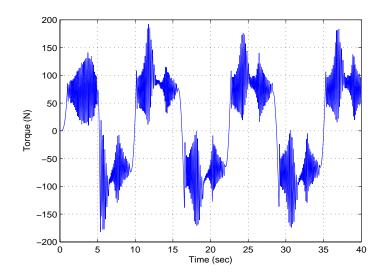
Figure 3–16: Torque input by the PD controller.
