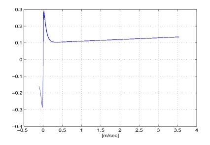
Figure 2–17: Friction coefficient vs slip velocity.
