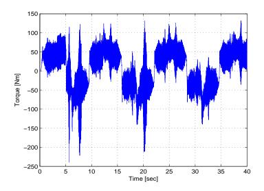
Figure 3–17: Torque input by the model-based controller with friction feedforward terms as described in (3–40).
