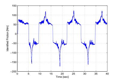
Figure 3–19: Identified friction from the adaptive term in the proposed controller.
