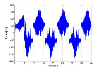
Figure 3–21: Torque input by the proposed controller when the circular disk was lubricated.
