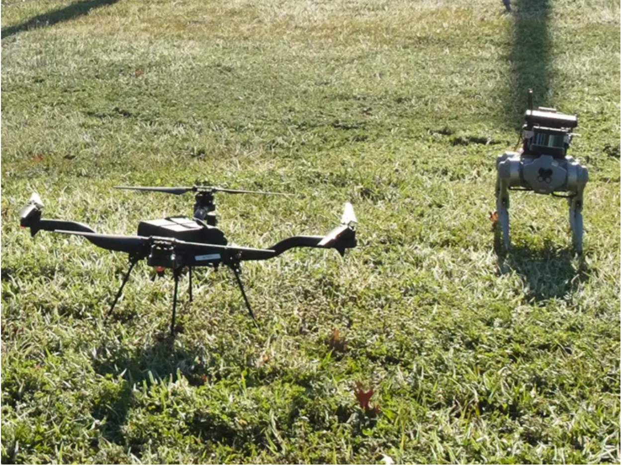
Figure 3-4. The Freefly Astro quadcopter (left) was used as the pursuer agent and the Unitree Go1 quadruped (right) was used as the target agent. The quadruped uses an Emlid RS+ RTK GPS for precise position updates, which is fused with attitude and heading data from a Microstrain 3DM-GX5-AHRS using the ROS2 robot - localization package.
