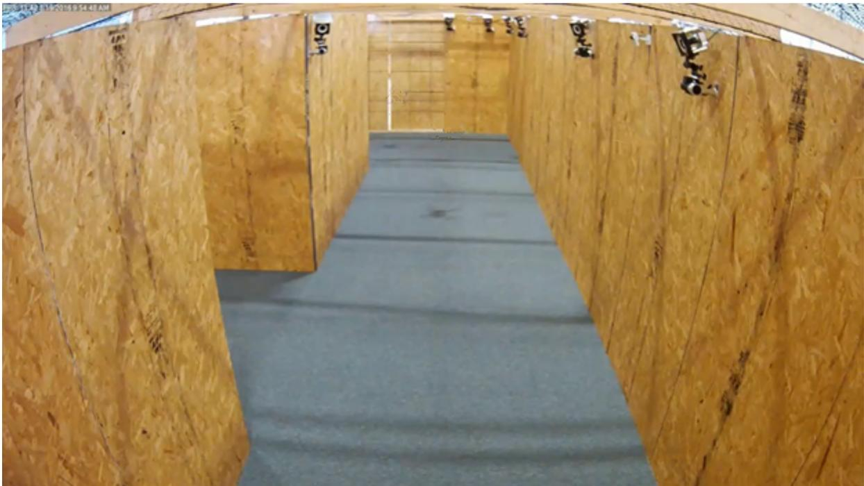
Figure 4-2. Photo courtesy of author. Image of a section of the wooden hallways in the environment and locations of the motion capture cameras in that section. The motion capture cameras were located throughout the environment attached to the upper portion of each wall.
