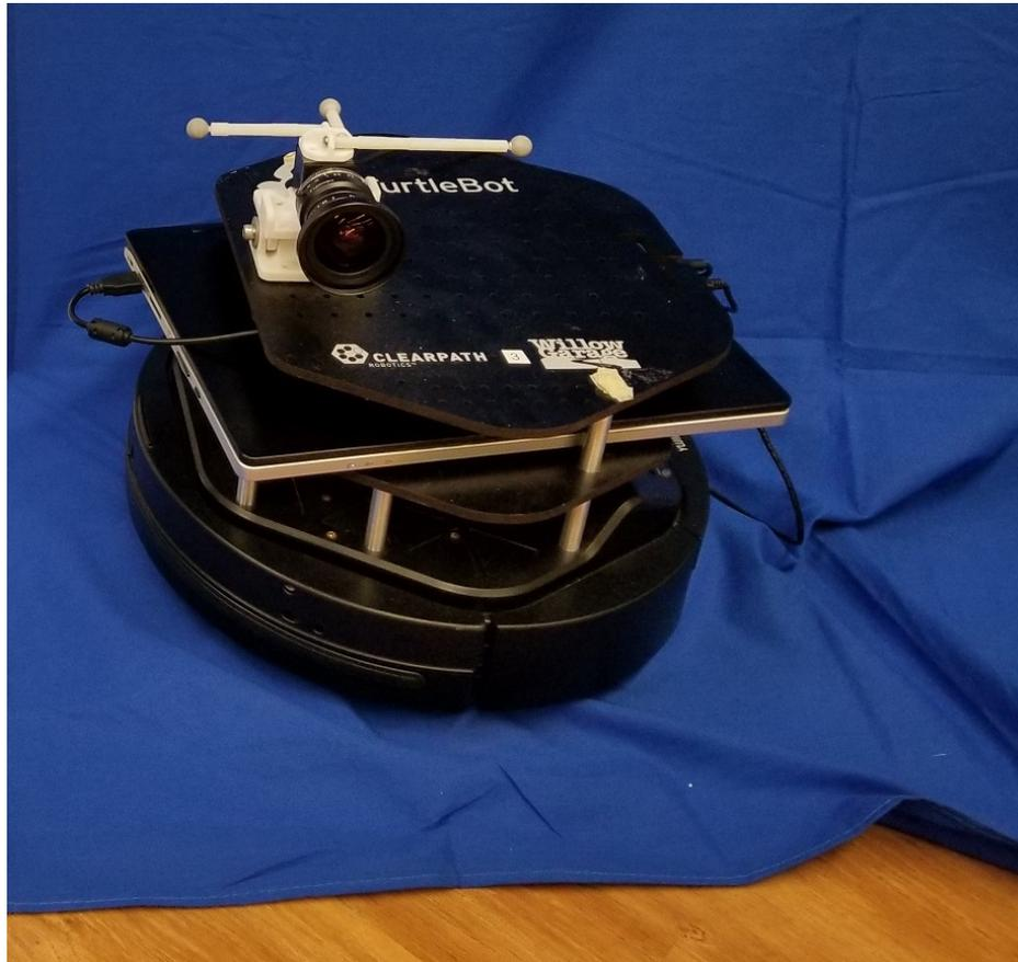
Figure 4-1. Photo courtesy of author. Image of the Kobuki Turtlebot and iDS uEye camera used for experiments.
