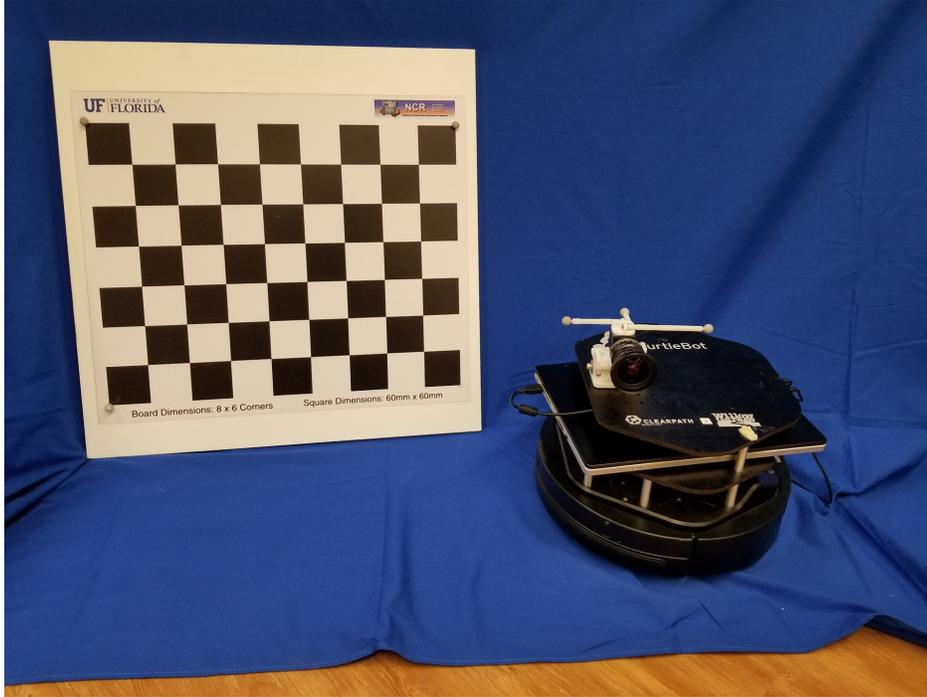
Figure 3-1. Photo courtesy of author. Image shows the checkerboard, Kobuki Turtlebot, and an iDS uEye camera used for experiments.
