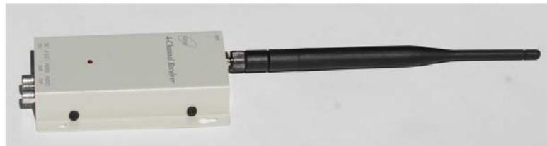
Figure C-1: RX-2410 2.4 GHz Wireless 4-channel Audio/Video Selectable Receiver
