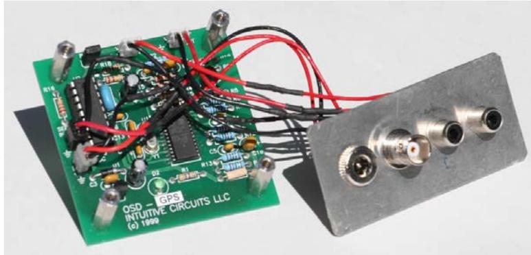
Figure B-4: Intuitive Circuits, LLC - OSD-GPS Overlay Board
