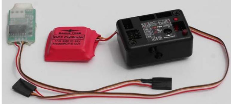
Figure B-6: Eagle Tree, Seagull, Wireless Dashboard Flight System - Pro Version: (1) Wireless Telemetry Transmitter, (2) Eagle Tree Systems G-Force Expander, and (3) Eagle Tree Systems GPS Expander
