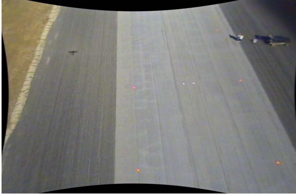
Figure 4–14: Single video frame from second flight test experiment with the lens distortion removed.
