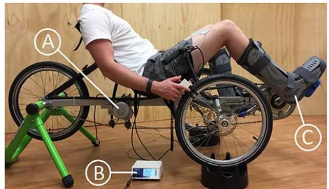
Fig. 2. Motorized FES-cycling test bed. (A) Electric motor. (B) Stimulator. (C) Orthotic pedals.
