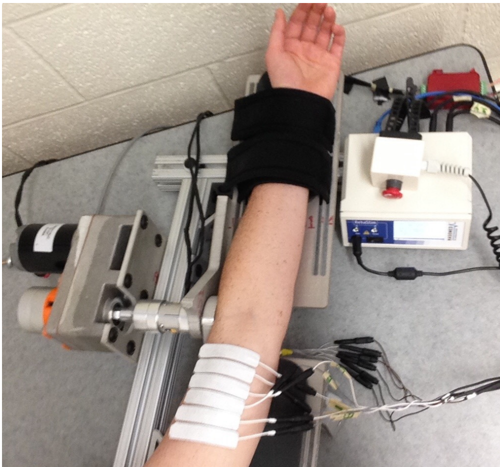
Figure 2. Six electrodes connected to a stimulator are evenly spaced on a participants biceps brachii. The participant's elbow joint is aligned with the motorized testbed's joint axis. An emergency stop button is provided for participants to voluntarily stop the test at any time.
