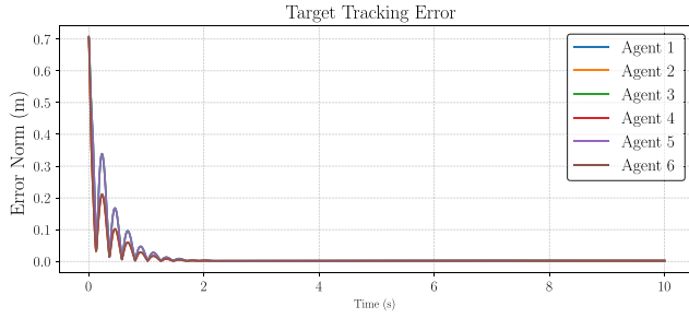
Fig. 3. Plot of the tracking errors for each agent, when the dynamic parameters a_i, b_i, c_i, d_i are selected from the uniform distribution U(0, 2.5) .
