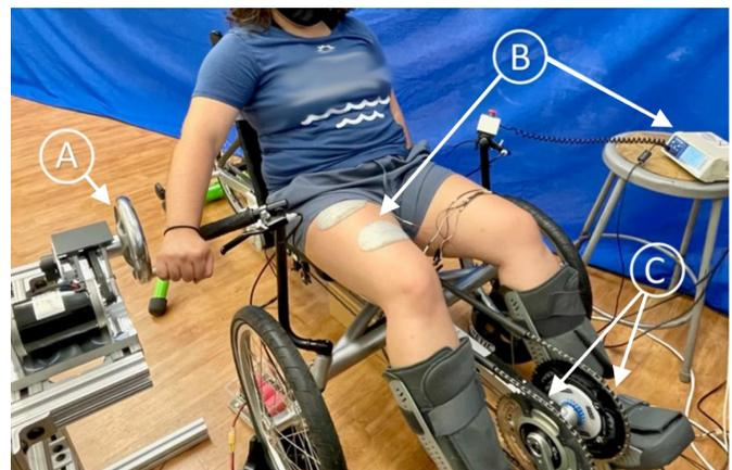
Fig. 2. Rehab-by-wire style teleoperated FES-actuated split-crank rehabilitation system, where the desired position and cadence are set by the user-operated hand-cycle marked by the letter A. The stimulation unit and dermal stimulation pads are marked by the letter B. The split-crank recumbent cycle crank sets are marked by the letter C.
