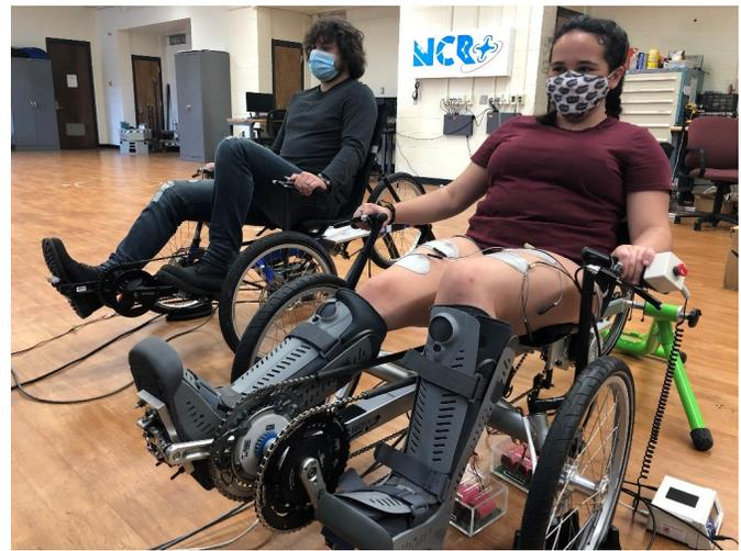
Fig. 1. Remotely operated FES-actuated split-crank telerehabilitation system shown in the foreground, where the desired position and cadence are set by a separate operator on a single-crank recumbent cycle shown in the background. Forward rotation of the crank arm, subsequently referenced in the control development, is that which would produce forward movement of the cycle if it were not stationary.
