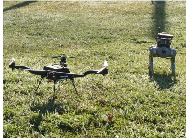
Fig. 4. The Freefly Astro quadcopter (left) was used as the pursuer agent and the Unitree Go1 quadruped (right) was used as the target agent. The quadruped uses an Emlid RS+ RTK GPS for precise position updates, which is fused with attitude and heading data from a Microstrain 3DM-GX5-AHRS using the ROS2 robot – localization package.
