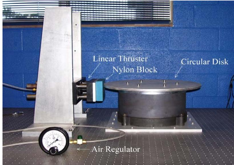
Figure 2-21: Testbed for the experiment.
